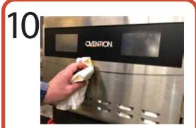
Polish and clean the exterior of the oven with a commercial-grade stainless steel polish.
