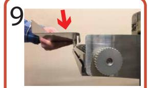
Replace each of the two jet plates, two air filters, two crumb trays and two end stops.
