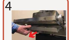
Remove crumb trays and end stops on both wings. Wipe down or wash as needed (dishwasher safe).
