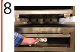
Spray rag with cleaner\* and wipe debris out of the cavity. Clean the inside of the door.
