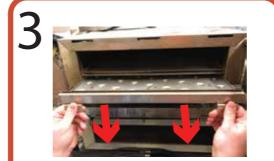
Open the oven door and remove top and bottom jet plates.
