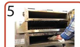
Spray rag with cleaner\* and wipe debris out of the cavity. **NEVER** spray directly into the oven.
