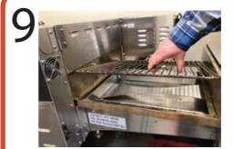
Replace each of the two jet plates, two air filters, two crumb trays and racks.
