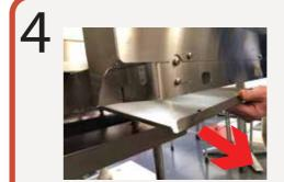
Remove crumb trays and racks on both wings. Wipe down or wash as needed (dishwasher safe).
