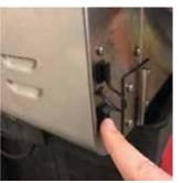
Turn off the oven with the rocker switch. When the oven is cool, the screens will read 'READY TO CLEAN'.
