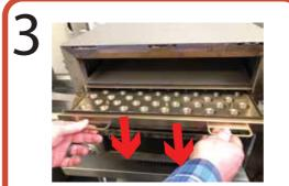
Open the oven door and remove top and bottom jet plates.
