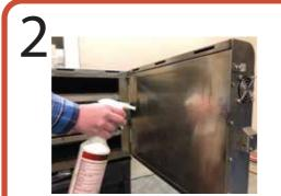
Using a non-caustic degreaser\*, spray the inside of the front door and wipe clean.
