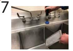
Using hot water and soap, gently rinse all air filters. Allow them to air dry completely before reinstallation.
