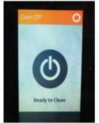
Turn off oven by touching the power symbol. Wait for the cooling fans to shut off, and for the screen to display "Ready To Clean"
