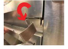
Remove and clean the drip tray. Lift up the tray, tilting the bottom outwards to release the tabs. Spray and wipe down as needed.
