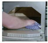
Wipe all interior surfaces of oven caviity, including door. DO NOT SPRAY INTO CAVITY. Wipe oven chamber using a dry, non-abrasive cloth.
